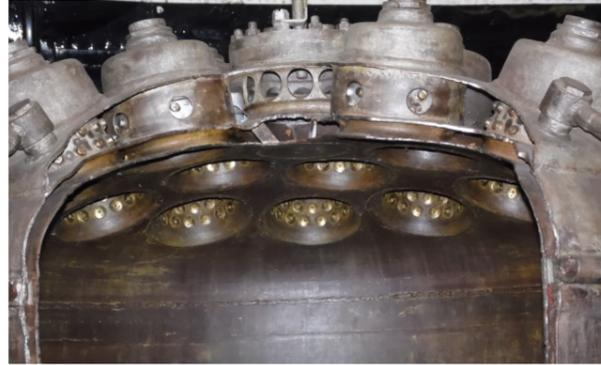
Detail of the A4's rocket engine showing the multitude of injection chambers and double wall construction.
