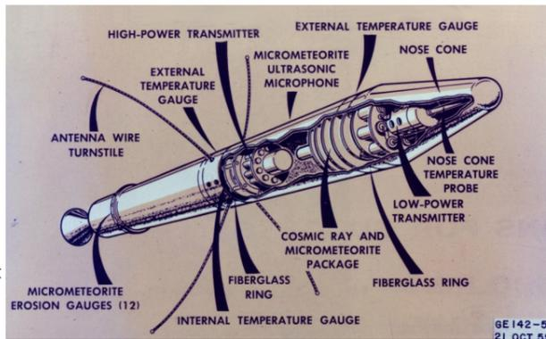
Schematics for „Explorer 1“, the first satellite successfully launched by the USA. Credit: NASA
