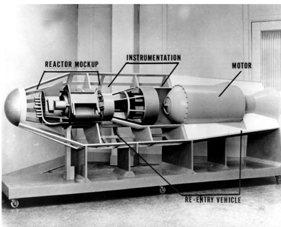
Mockup of the fourth stage of the Scout launch vehicle which launched the re-entry vehicle, including a reactor mockup, for AEC's Re-entry Flight Demonstration-1 (RFD-1) from Wallops Island, Virginia. 1963
